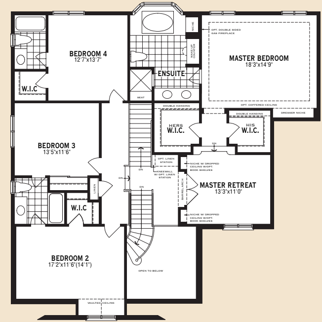
Opt. Second Floor Plan With 4 Bedrooms And 3 Baths With Master Retreat (Only Available With Optional Ground Floor Plan) (3796 Sq. Ft. Including 152 Sq. Ft. O.T.B.)
