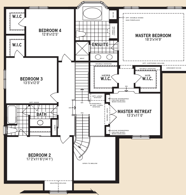
Opt. Second Floor Plan With 4 Bedrooms And 2 Baths With Master Retreat (Only Available With Optional Ground Floor Plan) (3796 Sq. Ft. Including 152 Sq. Ft. O.T.B.)
