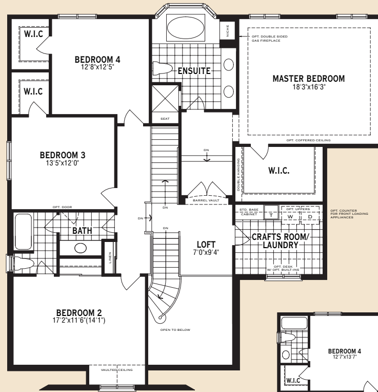
Second Floor Plan 4 Bedroom With 2 Bath (Only Available With Standard Ground Floor Plan)
