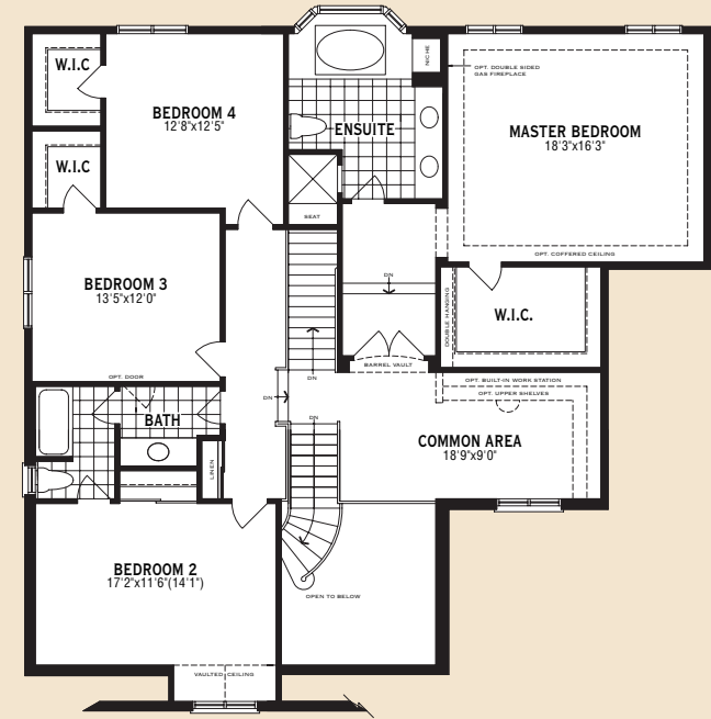
Std. Second Floor Plan With 4 Bedrooms And 2 Baths With Common Area For Optional Ground Floor Plan (3796 Sq. Ft. Including 152 Sq. Ft. O.T.B.)
